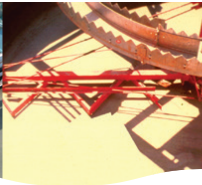
Common header pipe in the direct removal (DR) design
