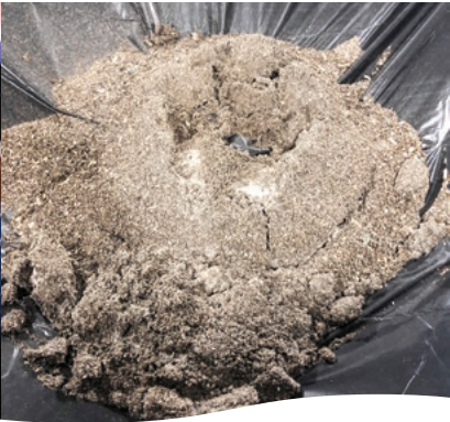
Discharged grit is typically 90% dry weight or greater. Organics are typically less than 10%.
