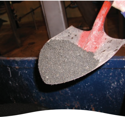
Discharged grit is typically 90% dry weight or greater. Organics are typically less than 10%.
