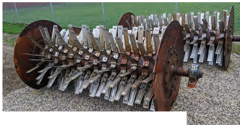
ABOVE: The Lakeside rotors at the Turkey Creek plant sustain high populations of microorganisms. LEFT: Mechanisms in the Lakeside clarifiers move solids to the center for the tank floor.
